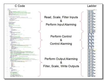
In the early days of industrial automation, programming was flat. We read the inputs, scaled the inputs, generated alarming on the inputs, performed the control algorithms to generate outputs, performed alarming on the outputs, scaled the outputs, and wrote the outputs using memory mapped I/O. Later when Functions became available, we consolidated some of the duplicate code, but the process was still essentially flat.
