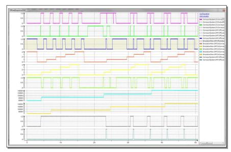
A Trace can be used to monitor the results of the simulation. And/or the simulation models themselves can monitor for the expected behavior in a fully automated test system. In this case, the traces show the handshaking between each piece of equipment, the outputs of the proximity sensors, the inputs to the motors, and the status of each conveyor simulator.
