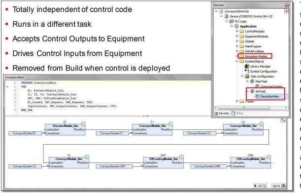
The simulation code often mirrors the control code. Here is the simulation code for the container handling system described earlier in this chapter. It contains the same blocks as the control code, except this is using the simulation
