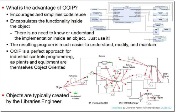
**Object Oriented** Industrial Programming (OOIP) simplifies the design of your plant or equipment and makes it much easier and more likely to reuse control objects on future designs. Your plant or equipment is made of objects (motors, actuators, sensors, etc.); the control for your plant or equipment should be too!
