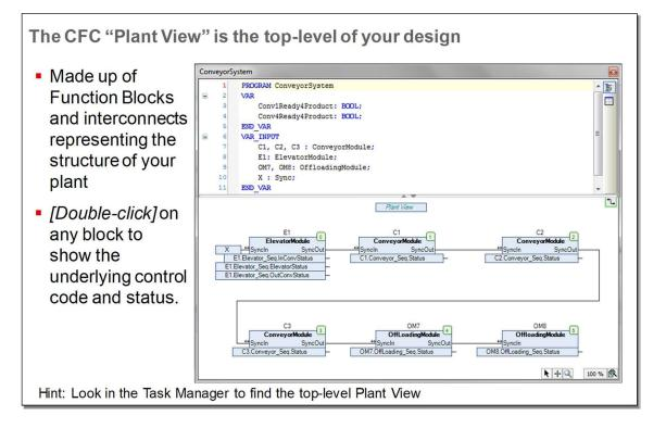
This graphic details the top-level of the material handling system described on the previous page. This is a blockdiagram of the plant. (Or this could be a block diagram of a section of the plant, since each level can stand on its own – there is no way to know (except in CODESYS the top-level is a Program and all other levels are Function Blocks.))
