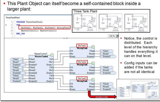
Again, the object of OOIP is to build completely selfcontained and selfreliant objects which can be used without any additional programming (such as adding its variables to a global variable list, or adding its alarms to an alarm manager, or adding its persistent variables to the Persistence Manager, etc.). Add the block into the design, connect its Program
