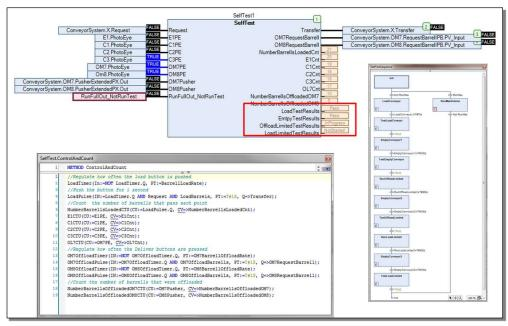
The simulation can be extended to include a full self-test of all the cornercases and unusual conditions of the control code. This is extremely helpful for future developers to test their modifications and verify that none of the existing operations were disturbed by the modifications.
