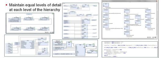
This author finds it far better to build a large design from a hierarchical arrangement of small and manageable blocks, than to build one large flat design. A well-designed hierarchical design consisting of logically partitioned blocks is much easier to understand, debug, and validate than one large flat design. This author typically limits the size of a building block to one page (or two pages with
