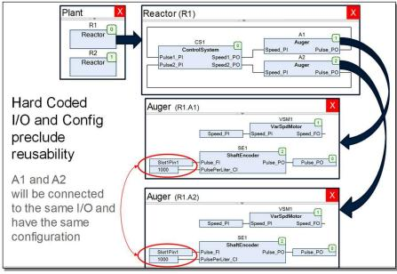
This figure shows how Abstraction, Composition, and Interfaces can be used to build a hierarchical process plant. At the top level, the Plant Program instantiates two Reactor objects, each of which have abstracted away the complexity of two Auger objects which themselves instantiate Motor and Shaft Encoder objects. The Shaft Encoder and Motor objects encapsulate all the functionality required to receive pulses from the shaft encoder and control the motor.
